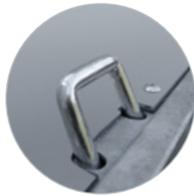
8 fixed tie hooks on the steel floor
