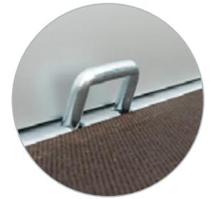
8 Tie hooks on the edge of the loading floor
