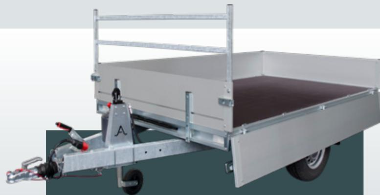
The ladder rack is the number one KLT accessory. It offers more mounting options and increases load protection.
