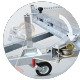
In length adjustable and rotatable winch
