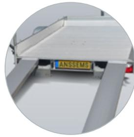
Aluminium ramps in integrated ramp holders
