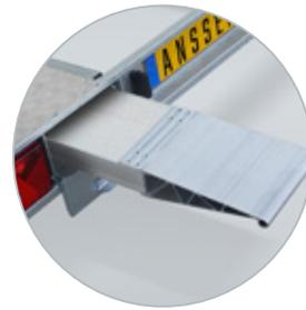
Aluminium ramps in integrated ramp holders
